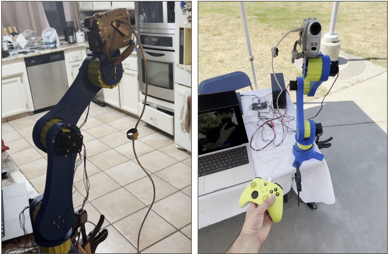
Figure 1. Left: the arm during the five-day build, joints assembled and under test. Right: on the table at club rush, driven from the Xbox controller.
